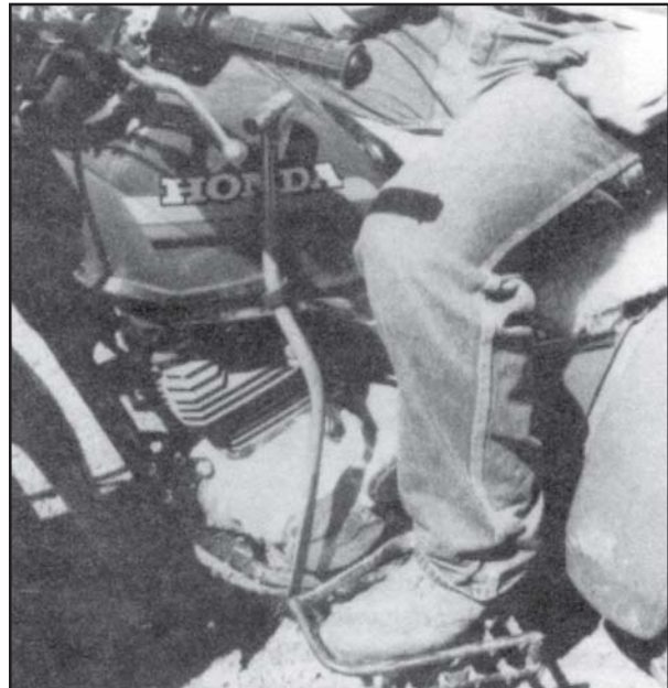
Figure 18. Hand controls can be utilized to safely shift foot-controlled gears on an ATV.
