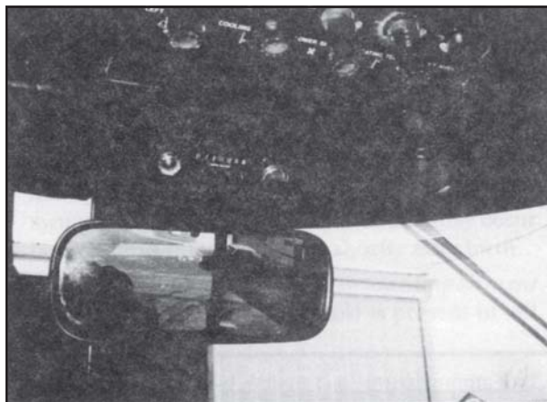
Figure 19. Large rearview mirrors with wide fields of vision are available which reduce the operator's need to turn around.
