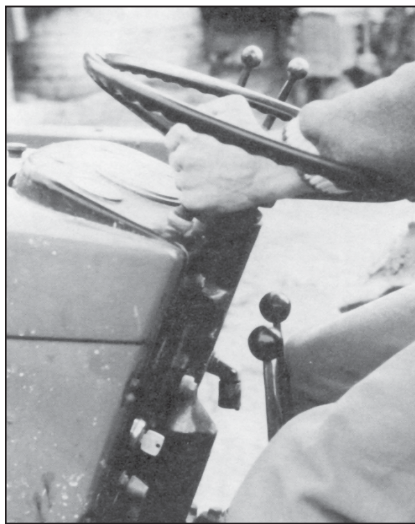
Figure 6. A push button stand switch eliminates the occurrence of breaking ignition keys due to Paul's difficulty in controlling movement.
